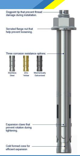
Hobson Tygabolts® are pre-assembled single unit wedge type anchors that are used in solid concrete applications. Fixing is achieved by controlled torqueing of the nut which draws the cone section up into the sleeve, thereby expanding it outward and forcing the Tygabolt™ against the sidewall of the pre-drilled hole.
